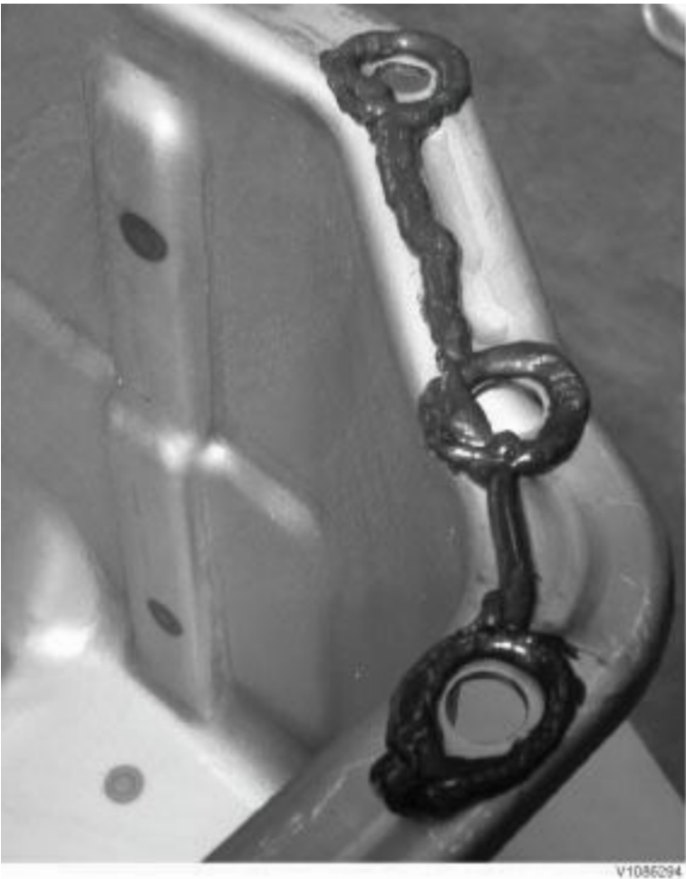
Figure 3 Sealing compound on oil sump
