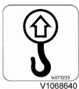
Figure 2 Point for lifting
