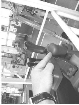
High speed travel switch on the dozer lever
