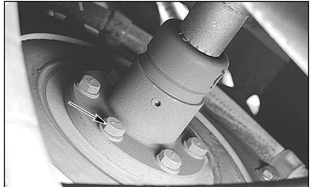
Remove the drive shaft bolts from the flywheel. Move the drive shaft clear of the flywheel.
