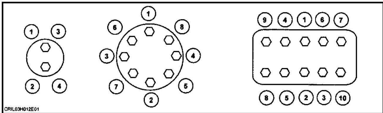
**NOTE:** Shown above is the suggested initial torque tightening sequences for general applications, tighten in sequence from item 1 through to the last item of hardware.
