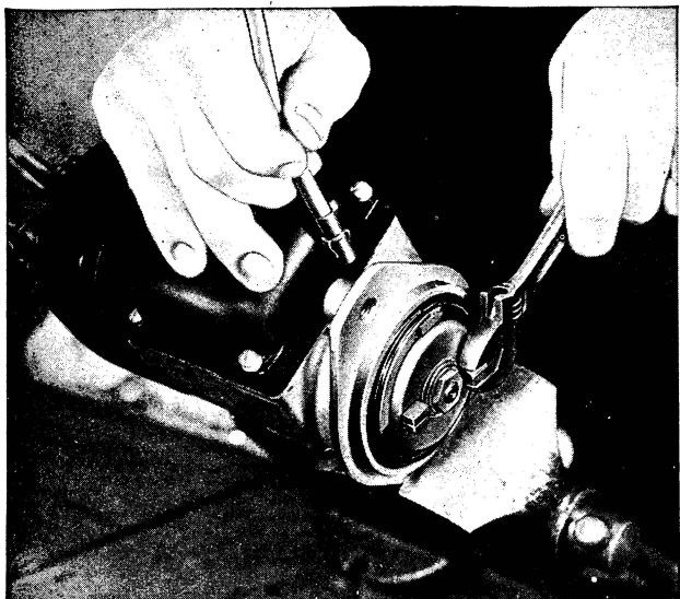
Figure 20. Locating Number 1 Firing Position on Magneto
