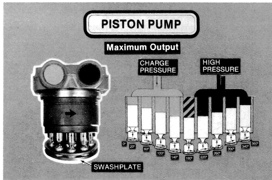
When the swashplate is tilted from the zero position, the pistons follow the swashplate surface, admitting oil until each piston reaches its maximum "down-stroke". As the pistons revolve past the maximum volume position, the inlet port is cut off and the discharge port is un-
