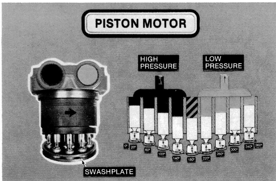
Where revolving pistons in the pump follow the "ups and downs" of the variable swashplate to displace fluid, in the motor, pressure on the pistons forces them to slide "down" the fixed swashplate, causing the piston block to revolve. With nine pistons in the motor, at any instant four are
