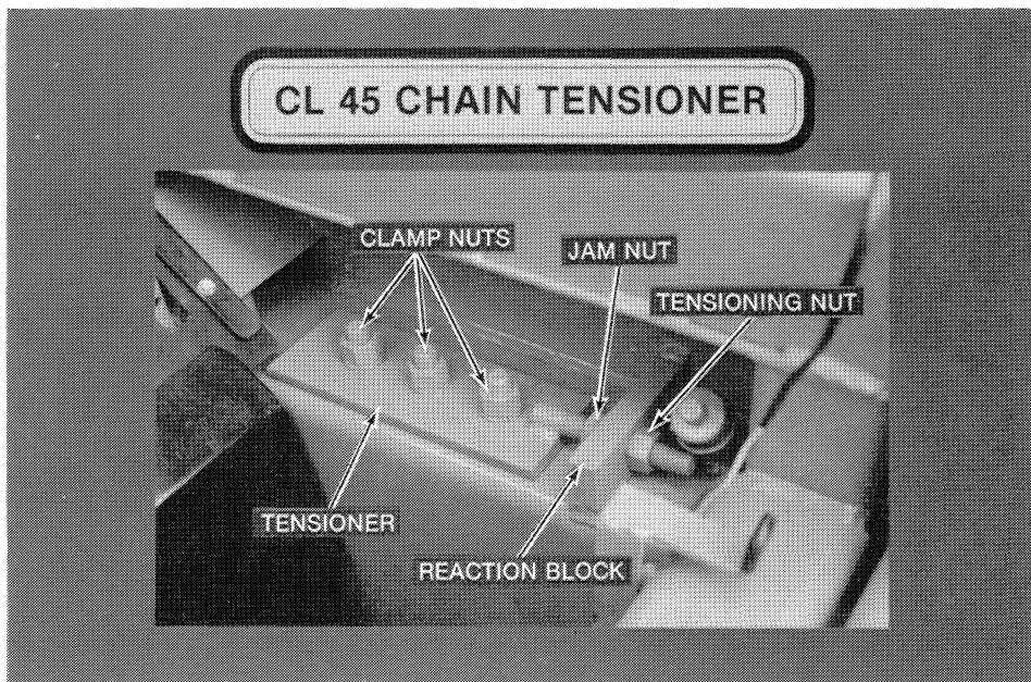
To adjust chain tension, three clamp nuts on the tensioner must be loosened, just enough to permit fore-and-aft movement. The jam nut at the rear of the reaction block must be backed off and the front nut
