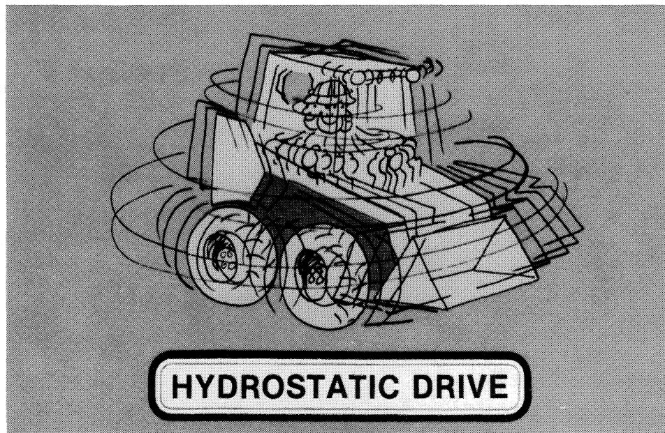
One feature all models have in common is hydrostatic drive, permitting infinitely variable speed control forward and reverse. Separate drive systems power left
