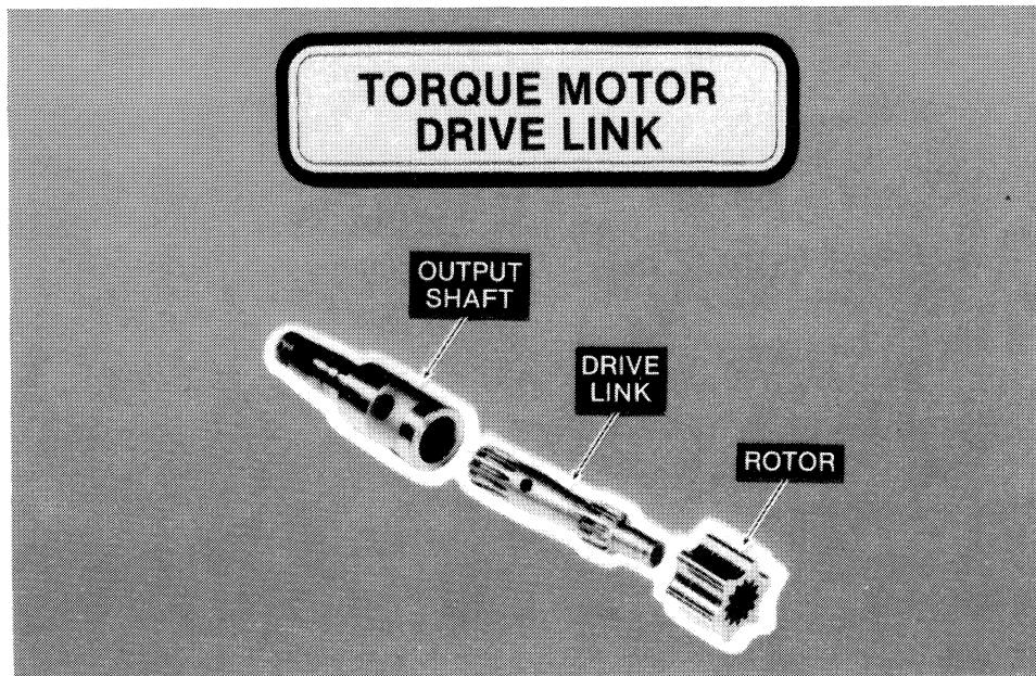
Splines on the drive link between rotor and output shaft are barrel-shaped to accommodate the wobbling motion imparted by the eccentrically-running rotor. Then,
