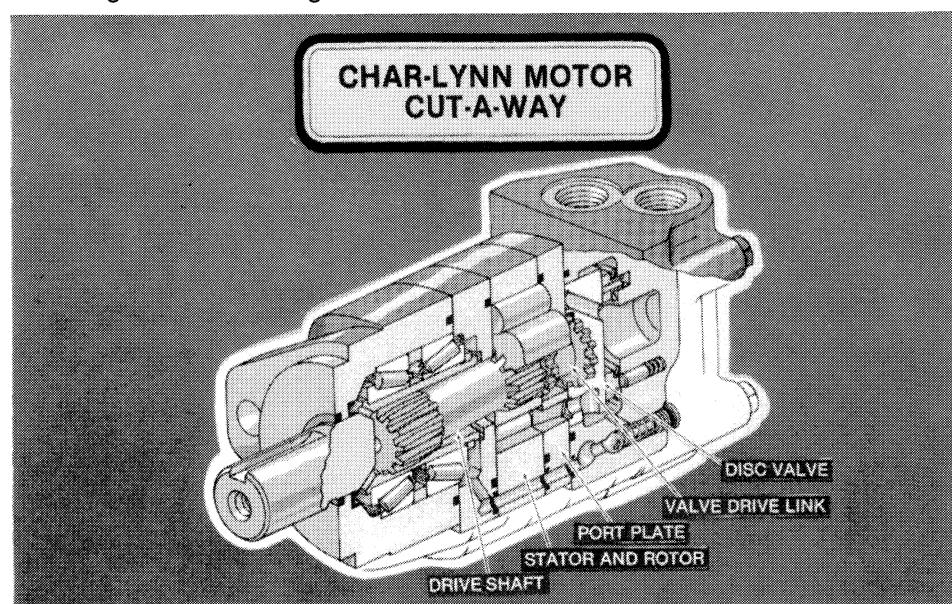
The Char-Lynn motor used in the CL-45 loader times the porting with a concentrically-rotating disc valve, driven by the rotor through a wobbling splined drive link. Though functionally similar to the
