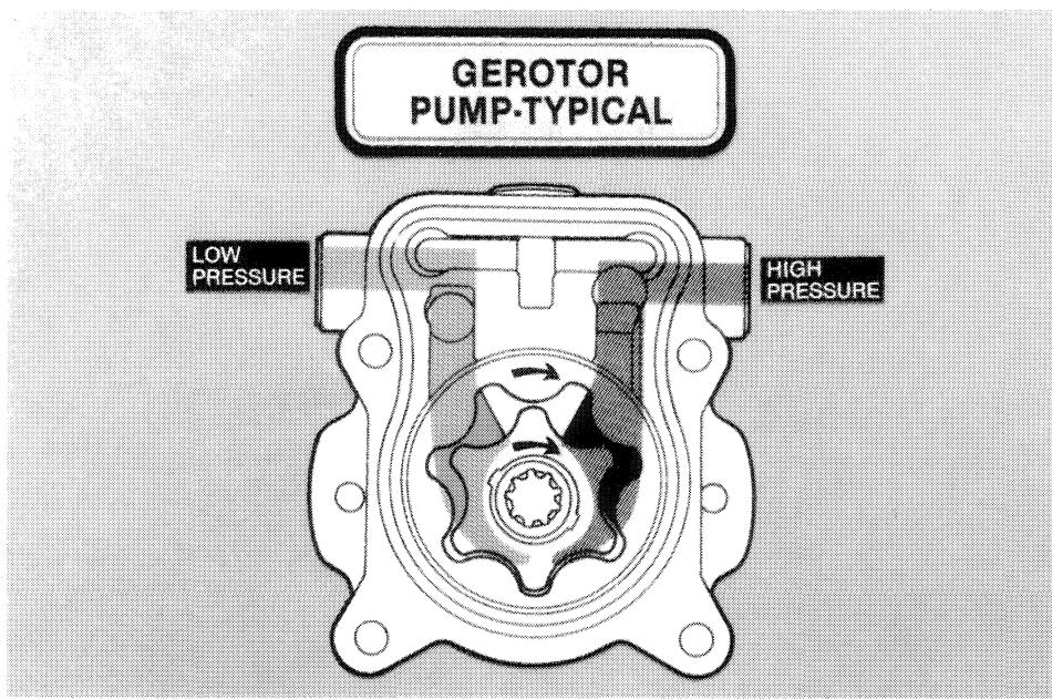
Like piston pumps, gear and rotor pumps will also function as motors. In the familiar type of rotor — or Gerotor — pump, each rotor rotates about its own center, but because the rotors are eccentric to each other the space between them is not uniform. An unequal number of
