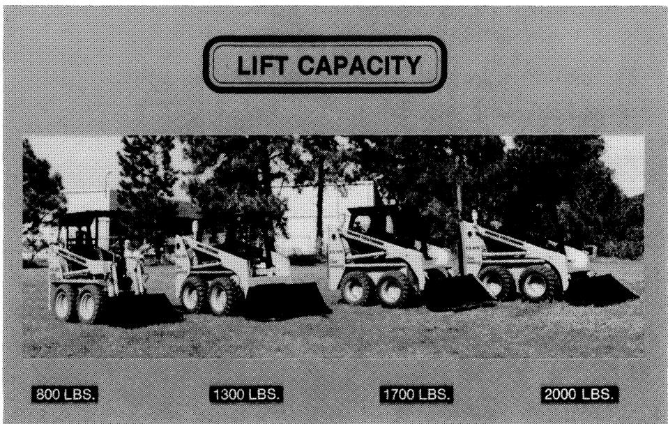
The differences between models are basically lift capacity and power ratings. Capacities are 800, 1300, 1700 and 2000
