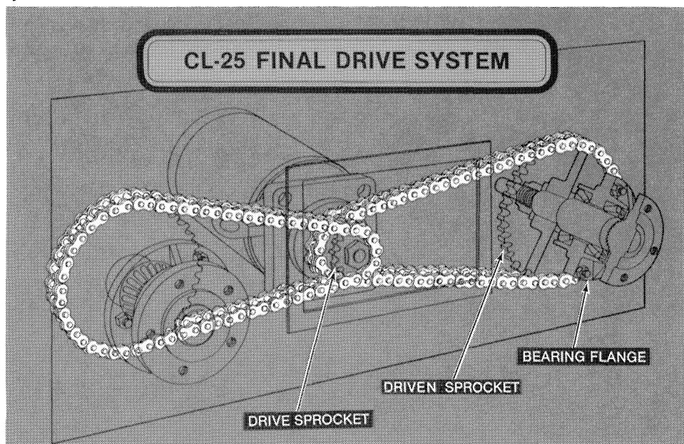
In the CL-25 two short chains connect the double drive sprocket, mounted on the motor shaft, to the axle driven sprockets. The bolt circles in the axle bearing flanges are eccentric to the bearing bores to permit adjusting chain tension at initial assembly. Because of the short chain
