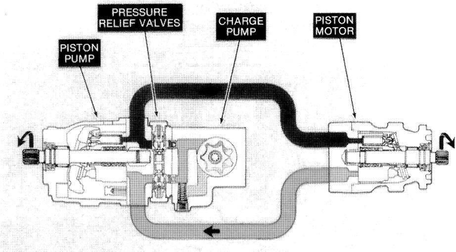
To understand the operation of hydrostatic drive motors, it may help to think of them as pumps with functions reversed. Instead of driving a shaft to displace and pressurize fluid, fluid under pressure is forced
