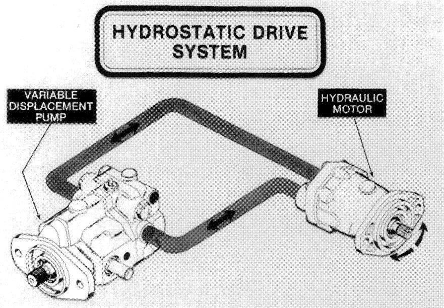
Each hydrostatic drive system consists of a variable-displacement pump capable of delivering oil at flow rates from zero to maximum in either direction, and a positive-displacement hydraulic motor con-
