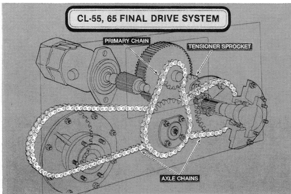
In the CL-55 and 65 final drive system, the axle sprockets are connected to the double drive sprocket by two relatively short chains. Half links are available to permit adjusting the length of the axle drive
