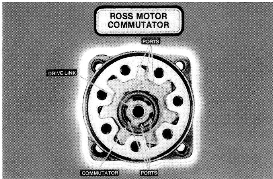
In the Ross torque motor, the porting is made to rotate with the rotor by a "commutator", which revolves eccentrically to cover and uncover ports to the expanding and contracting chambers. High and low
