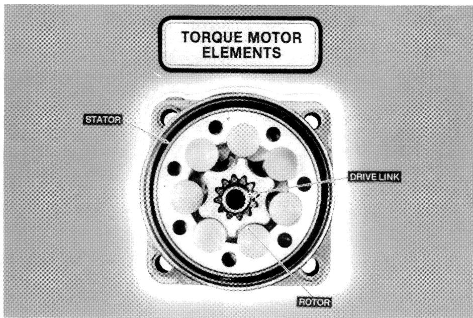
The rotor-type torque motors used in Ford compact loaders work much the same, but with a few mechanical differences. First, the outer rotor becomes a stator, and does not rotate. Roller vanes replace the fixed
