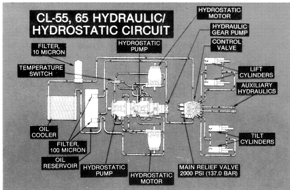
The rest of the hydraulic system serves the hydrostatic drive. When you pack this much plumbing into the limited space available in a compact loader, it gets to looking complicated, but the schematic helps in sorting it out. This is the CL-55 and 65 hydraulic system. It's repre-
