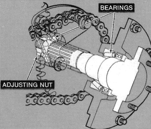
Axle bearing arrangement also varies from model to model. Tapered roller bearings are used in all cases. CL-55 and 65 bearings are straddle-mounted, with inboard bearing supports mounted in the chain
