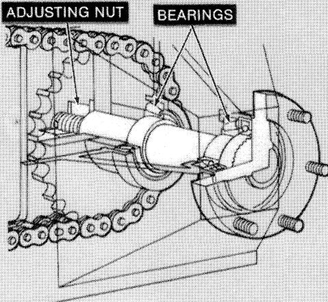
CL-45 axle bearings are also overhung-mounted, in bearing recesses built into axle housings projecting from the chain case outboard wall. Access to the bearing nuts is through removable cover plates on the inboard wall. Because of the increased outboard projection of CL-45 wheel flanges, CL-45 wheel discs are dished con-
