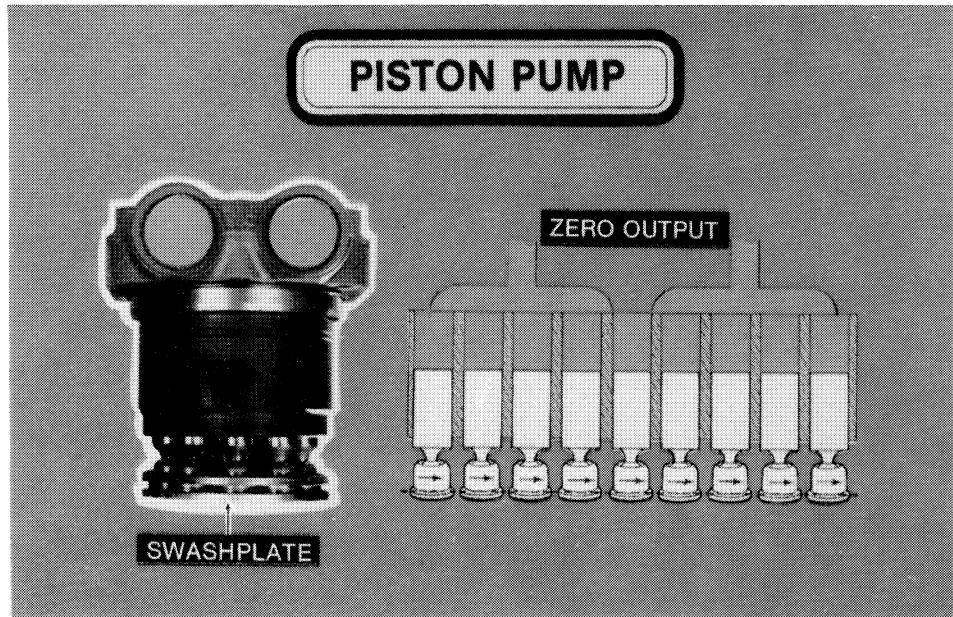
The hydrostatic drive pumps are of piston type, each containing nine pistons with ball-joint slippers revolving in contact with a tiltable "swashplate". The swashplate is in effect a variable cam which varies
