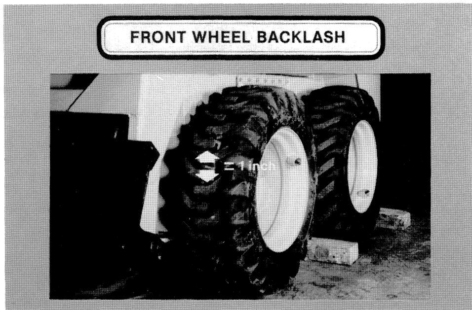
Therefore, routine tension checks are recommended for this model, after the first fifty hours and every 200 hours thereafter. Chain tension is checked by measuring front wheel backlash, with the front wheel
