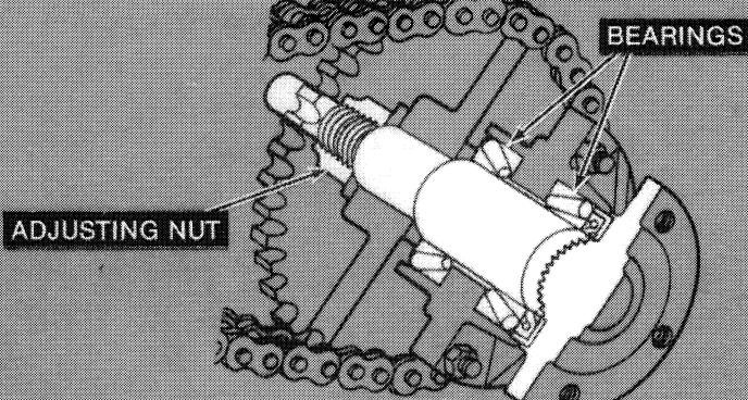
CL-25 axle bearings are overhung-mounted, in bearing flanges bolted to the chain case outboard wall. Removable covers on the inboard wall permit access to the bearing nuts for adjustment. The
