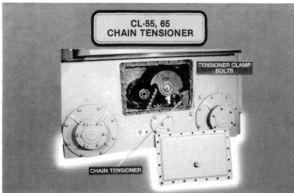
Two clamp bolts through the chain case outer wall lock the tensioner in position, and must be loosened for tension adjustment. When properly tensioned, the long span of the primary chain should deflect 1/2 to 3/4 inch. After adjusting, the tensioner clamp bolts should be torqued to 80 to 85 lbs.-ft.
