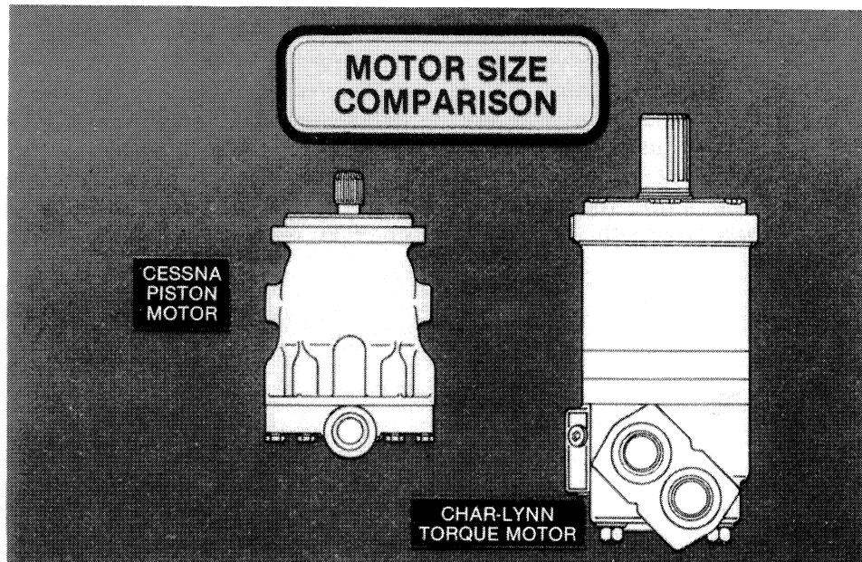
The differences between piston and rotor-type motors are considerable. Piston motors are smaller and lighter in weight for comparable power capabilities, reflecting their aircraft industry background. Compactness is desirable in compact loaders where space is at a premium, but
