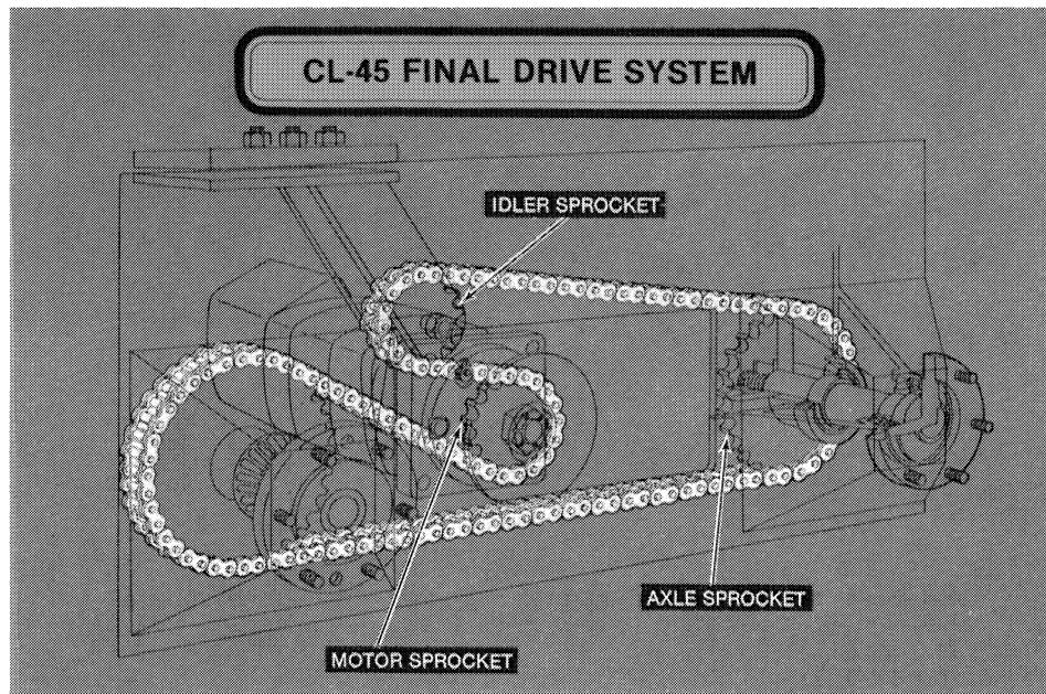
The CL-45 final drive system incorporates a single chain on each side connecting the axle sprockets and the motor sprocket, with an adjustable idler sprocket to control chain tension. Because the tensioner location is symmetrical side-to-side, and the drive motors are offset from each other fore-and aft, the right-side chain is
