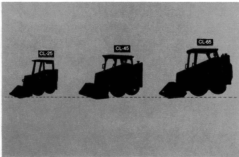
While there are dimensional variations from model to model, the four — eventually five — fall into three basic configurations, distinguished by drive pump and motor size and final drive layout. The CL-25 is by
