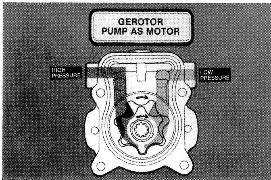
If used as a motor, high pressure oil would be admitted to the expanding chambers up to maximum volume, then the inlet port would be cut off and the outlet port opened.
