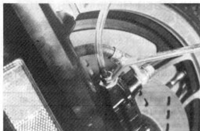
It is common for air to become "trapped" in the extra hoses or valves of the anti-dive system. Repeating the sequence of brake bleeding will remove most of this air. If the lever feel is still spongy after several bleeding sequences it may be necessary to remove the anti-dive modulator from the anti-dive assembly. This will allow the modulator to be "tipped" upwards, enabling the trapped air to be purged from the system.
