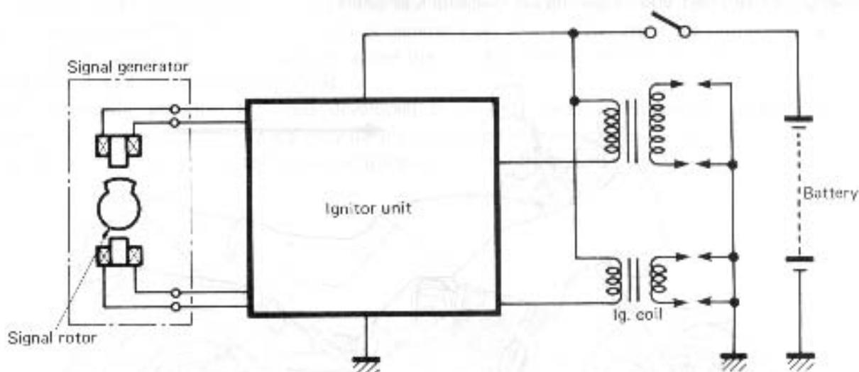
When the signal rotor is rotated in the system block diagram above, the signal "A" is generated in the pick-up coil. The thus-generated signal will be converted to the signal waveform "B" at the inside of the ignitor unit. Based on this "B" waveform, control is made by means of the advancing control circuit and the closing angle control circuit. As a result, the timing advance takes place, as shown in Fig. "C".
