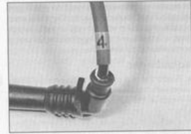
3.2d The plug wires (HT leads) are labeled according to cylinder number (counting from the left side of the motorcycle)
