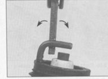
3.6b To change the gap, bend the side electrode only, as indicated by the arrows
