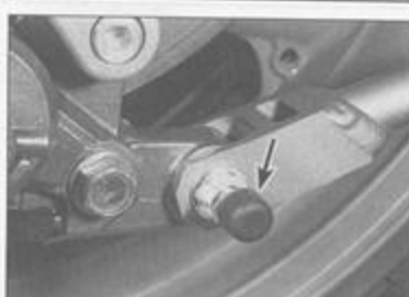
2.5 Remove the rubber cap (arrow) and the cotter pin (if equipped); loosen the nut on the torque link bolt
