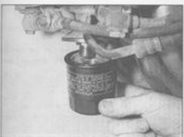
18.10b Coat the filter gasket with clean engine oil and thread the filter on (H1 model)
