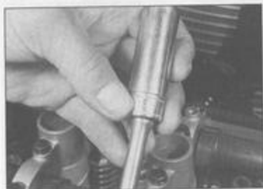
3.1 A 16 mm plug socket is required for spark plug removal
