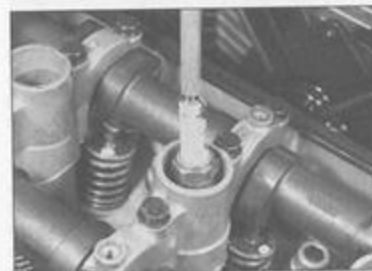
3.2f . . . a gripping tool like this can be used to pull the plug out of its bore
