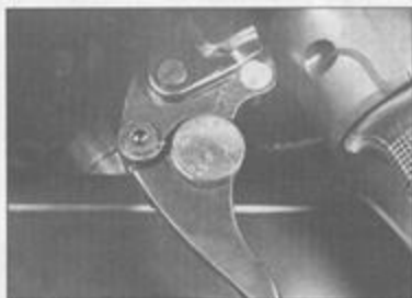
10.1 Turn the span adjuster to change the clutch lever distance from the handlebar
