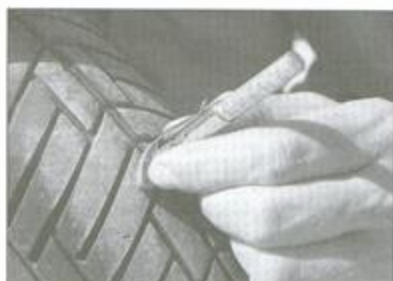
2 Measure the tread depth at the center of the tire using a tread depth gauge.
