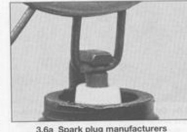
3.6a Spark plug manufacturers recommend using a wire type gauge when checking the gap
