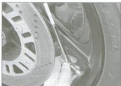
1 Check the tire pressures when the tires are cold and keep them properly inflated.
