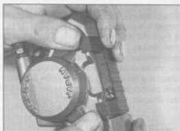
9.3 Remove the pad cover (if equipped) from the rear caliper to inspect the pads
