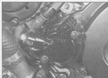
10.2 Look for fluid leaks around the clutch release cylinder and make sure its mounting bolts are tight
