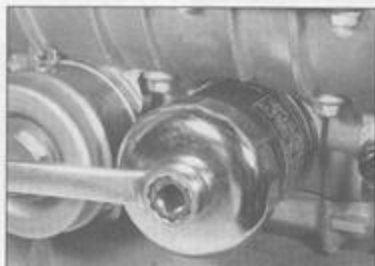
18.7a Unscrew the oil filter with an oil filter wrench; the square opening allows a torque wrench to be used for installation . . .
