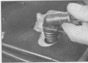
3.2a Rotate the plug caps back and forth to break the seal . . .
