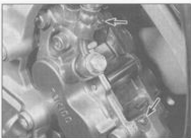
9.2a Remove the screws (arrows) and lift off the pad spring to inspect the front brake pads
