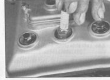
3.2e If the spark plug didn't stay in the wrench rubber insert, lift it out once it's loose . . .
