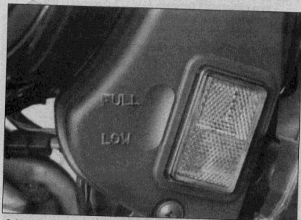
3.15 Check coolant level through the inspection hole in the right side cover; it should be between the Full and Low marks with the engine cold
