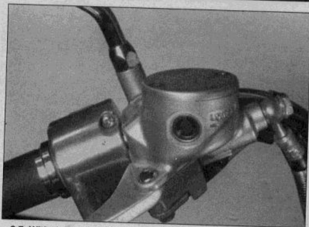
3.7 With the master cylinder in a level position, check the fluid level in the inspection window
