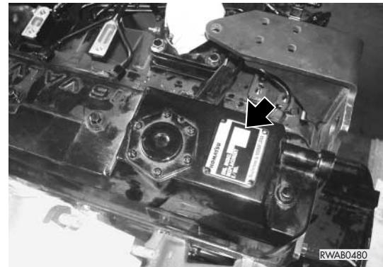
The plate regarding the exhaust emission regulations is applied to the front side of the tappet cover.
