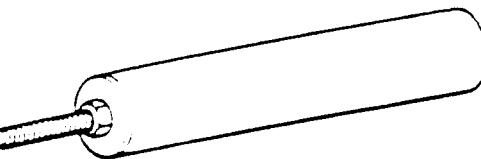
992/00800      Extractor for removing axle pivot pin
