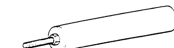
992/00800 Extractor for removing axle pivot pin
