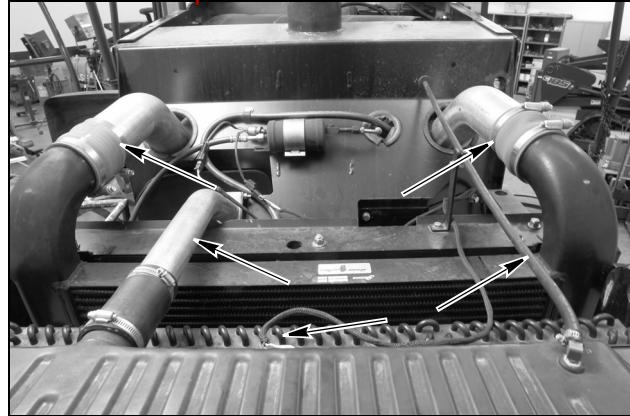
Loosen clamps and remove upper radiator hose and tube. Loosen the clamps and remove the hoses from the after cooler. Loosen clamp and disconnect radiator vent hose, disconnect cooling level sensor.
