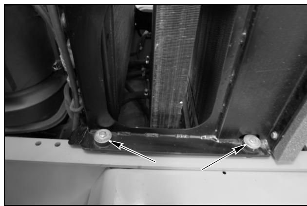
Remove the mounting bolts for the cooler pack.
