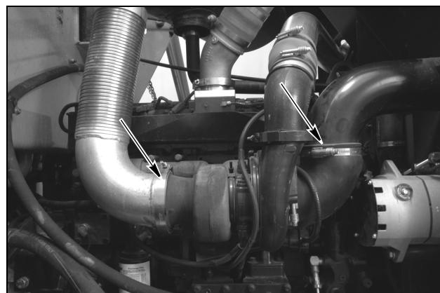
Loosen the hose clamps, disconnect the turbo inlet hose. Loosen the clamp and disconnect the muffler flex pipe from the turbo.
