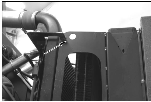
Attach lifting equipment to the lifting points on cooler pack.
