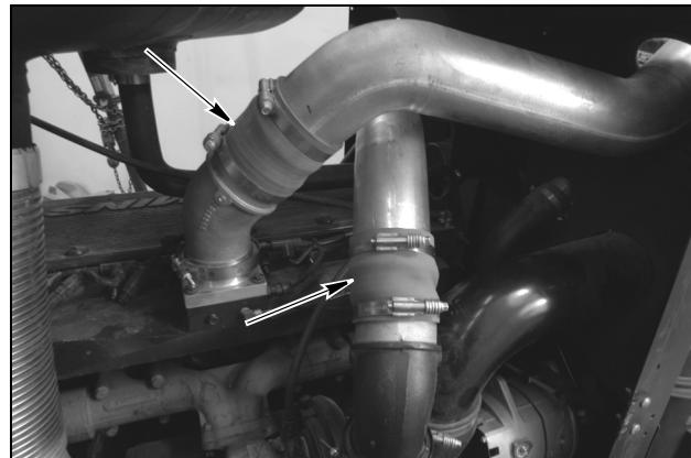
Loosen the hose clamps, disconnect and remove the after cooler tubes from the machine.
