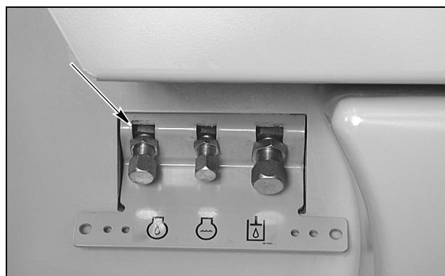
Put a container capable of holding at least 12.3 liter (13 U.S. quarts) below engine oil drain. Remove cap and drain oil into container. Install cap after oil has drained.
