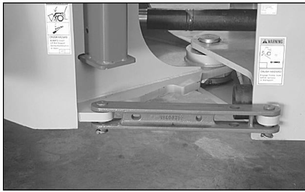
Park machine on a level surface and lower bucket to ground. Put articulation lock in LOCKED position.
