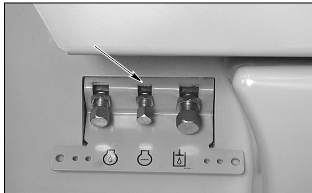
Put a container capable of holding at least 22.7 liter (6.0 gallon) below radiator drain. Remove radiator cap. Remove cap and drain coolant into container. Install cap after coolant has drained. Install radiator cap.
