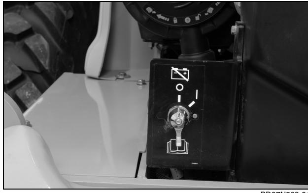
The master disconnect is located under the hood on the left rear side of the machine. Raise the hood put master disconnect switch in OFF position. Remove both battery covers and disconnect batteries from the machine.
