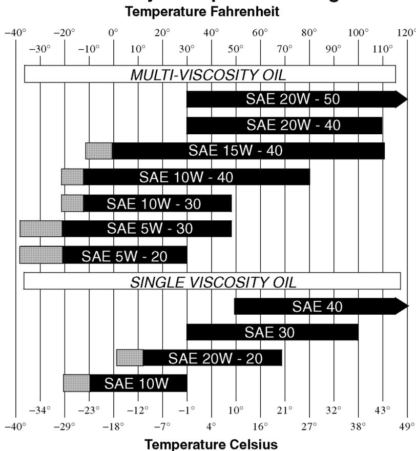
**NOTE:** Use of an engine oil pan heater or an engine coolant heater is required when operating temperatures are in the shaded area.
