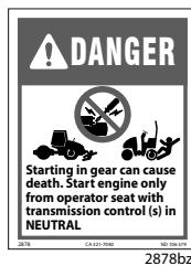
Starting in gear could cause death. Start the engine from the operator seat only with the transmission control(s) in neutral. Failure to comply will result in death or serious injury. (Symbol located on the hood)
