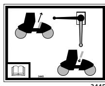
Pump to lift the hood. (Symbol located on the inner side of the disconnector door)
