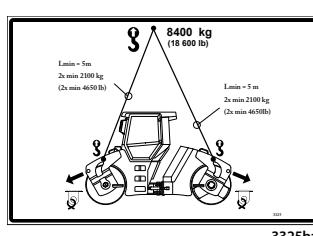
Use rigging of sufficient loading capacity to lift the Machine. Secure the Machine's joint before lifting. (Symbol located on the left side of the machine)
