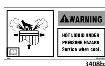
Do NOT open the expansion tank cap until the liquid cools down below 50°C (122°F). Failure to comply could result in death or serious injury. (Symbol located on the righthand side of the hood above the door)
