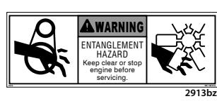
Maintain a safe distance from the rotating cooling fan, pulley and belt. Keep clear or stop engine before servicing. Failure to comply could result in death or serious injury. (Symbol located on the right side of the hood and on the cooler)
