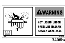
Do NOT open the expansion tank cap until the liquid cools down below 50°C (122°F). Failure to comply could result in death or serious injury. (Symbol located on the righthand side of the hood above the door)
