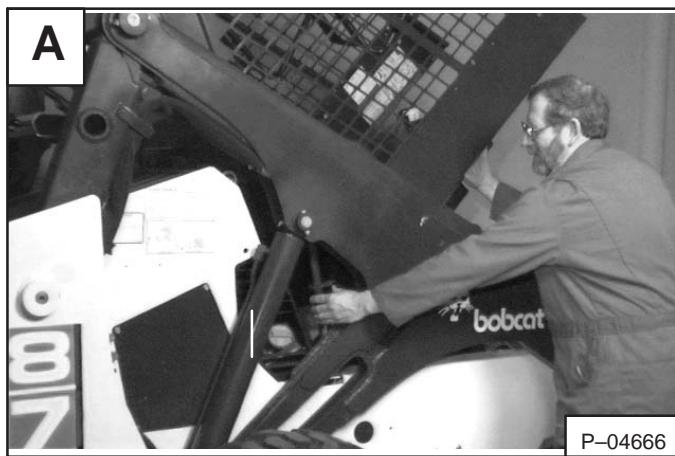
Release the latching mechanism (Item 1) [B] and pull the cab all the way down.
