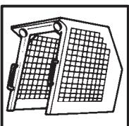
2. Check that ROPS mounting hardware is tightened and is Melroe approved.
