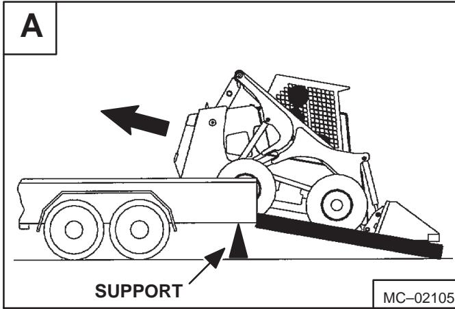
A loader with an empty bucket or no attachment must be loaded backward onto the transport vehicle [A].
