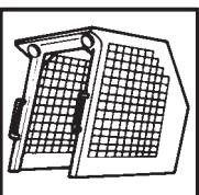
2. Check that ROPS mounting hardware is tightened and is Melroe approved.
