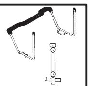
5. Check lift arm support device, replace if damaged.
