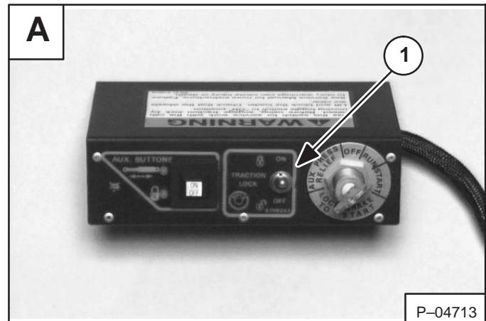
Move the traction lock override switch (Item 1) **[B]** to the OFF position so the traction function is unlocked. The wheels are now able to turn.
