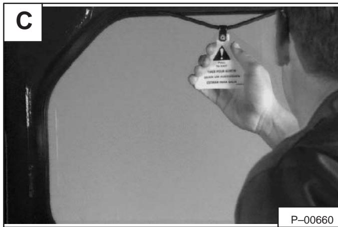
Push the rear window out of the rear of the operator cab.
