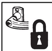
10. Bob-Tach wedges and linkages must function correctly and be in good condition.
