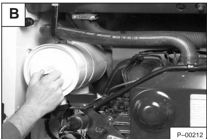
Remove the wing nut at the large air filter element [D].
