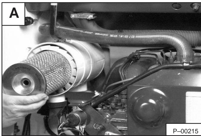
Only replace the inner filter element under the following conditions **[B]**.
