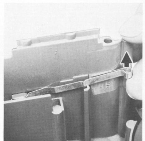
Bottom: Removing ignition stop switch
