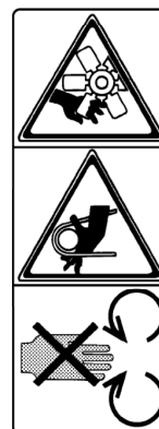
(3) Part No. K1213-6586-1 Stay clear of engine fan and fan belt.
