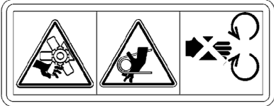
(4) Part No. K2581-6543-1 Stay clear of engine fan and fanbelt
