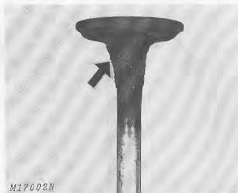
Fig. 5-Lead Deposits on Leaky Intake Valve
