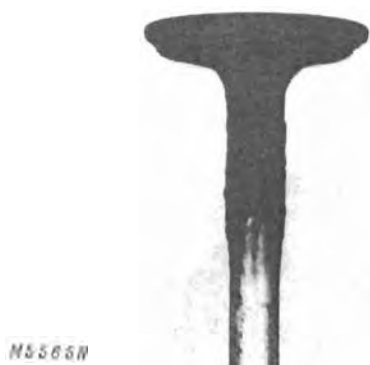
Fig. 5-Gummy Valve Causing Valve to Stick
