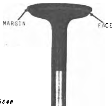
Fig. 4-Exhaust Valve Running Too Hot
