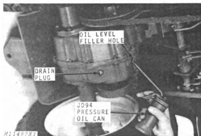
Fig. 3-Adding Oil to Transaxle
