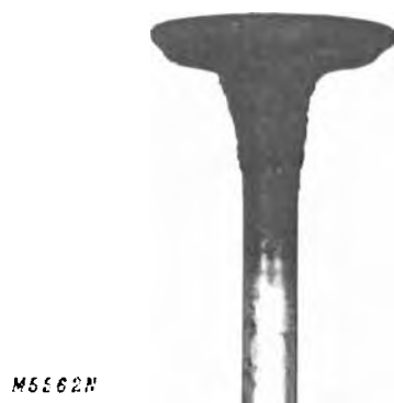
Fig. 2-Lead Deposits on Leaky Intake Valve
